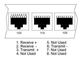
Figure 2-1. RJ45 Network Ports
